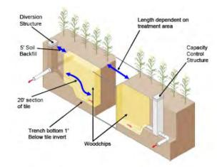
**Figure 4-30.** Denitrifying Bioreactor Diagram (*Source*: Richard Cooke, University of Illinois Urbana-Champaign)
