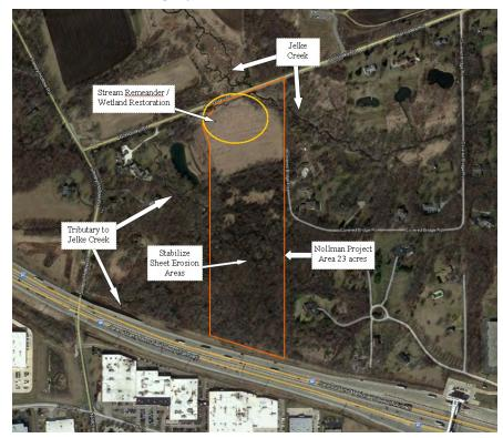
Figure 4-28. The 23-acre Nollman Parcel project area could include remeandering a tributary to Jelke Creek, as well as up to 2 or more acres of wetland restoration. In addition, upland (south) sheet erosion areas could be stabilized by replacing invasive shrubs with desirable, ground-stabilizing vegetation.
