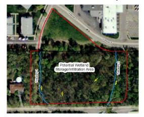
**Figure 4-27.** The Macintosh Creek Headwaters project would provide between 16 and 25 acre-feet of storage within restored wetlands. Runoff is currently discharged to the site from Meadowdale Mall to the north. (Source: Village of Carpentersville report prepared by AES)
